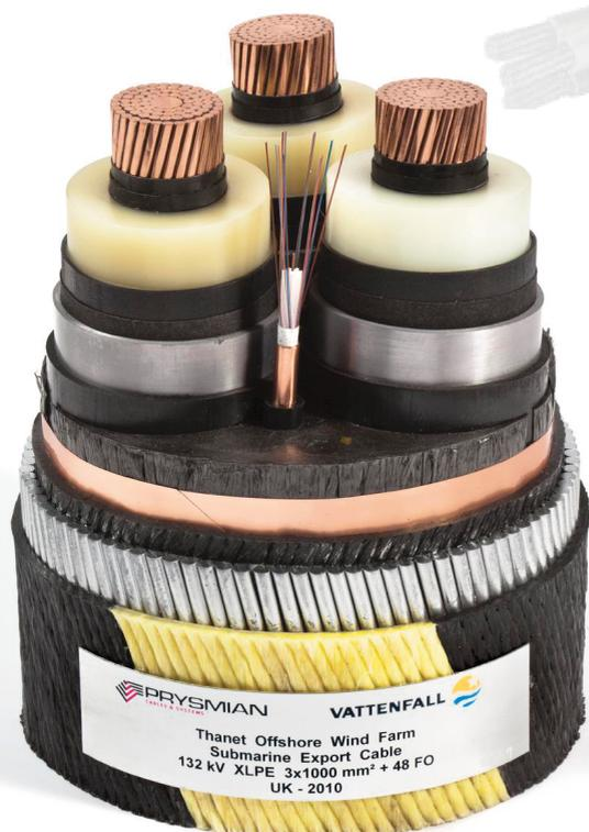
This recent 132kV XLPE submarine power cable could carry 180MW of power from an offshore wind farm to the UK national grid. Optical fibers provide a means of monitoring the cable's temperature.
