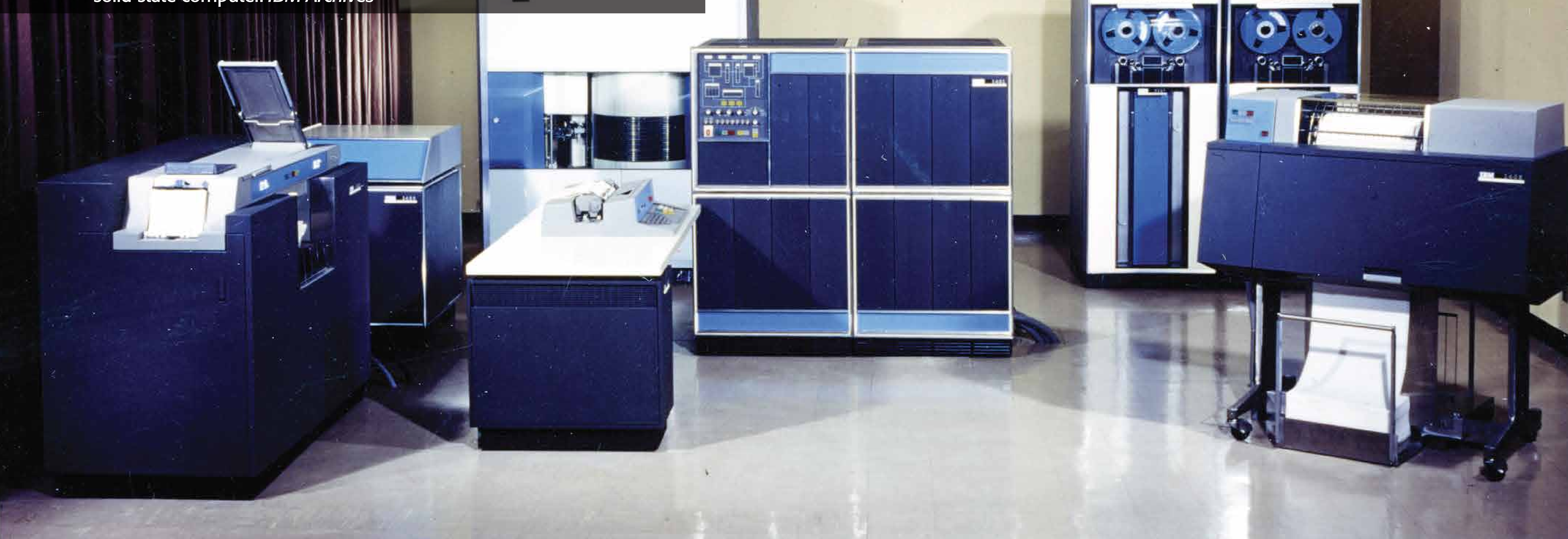
When IEEE was formed, the IBM1401 was the world’s most widely used solid-state computer. IBM Archives
